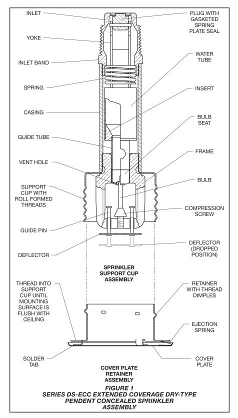
the glass bulb, and the bulb seat is released. The compressed spring is then able to expand and push the water tube as well as the guide tube outward. This action simultaneously pulls inward
