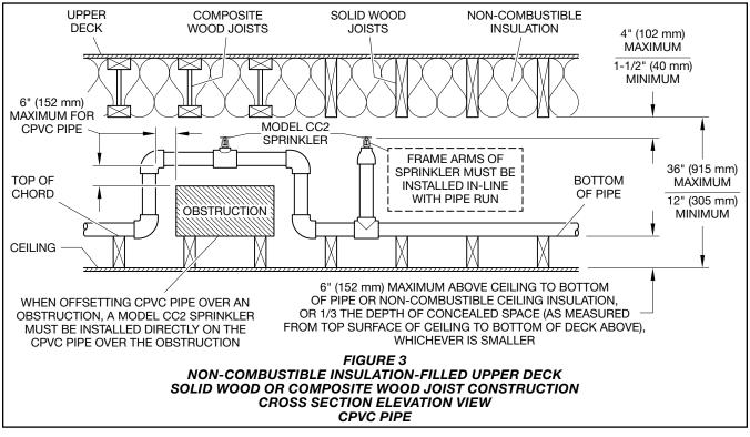
in. (305 mm) must be laterally braced using methods described in the NFPA standards.
