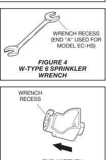
PUSH WRENCH IN TO ENSURE ENGAGEMENT WITH SPRINKLER WRENCHING AREA
