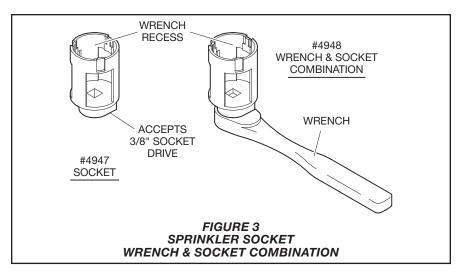
Sprinklers which are found to be leaking or exhibiting visible signs of corrosion must be replaced.
