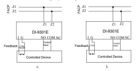
Below figure shows connection of the module to devices controlled by 24V
